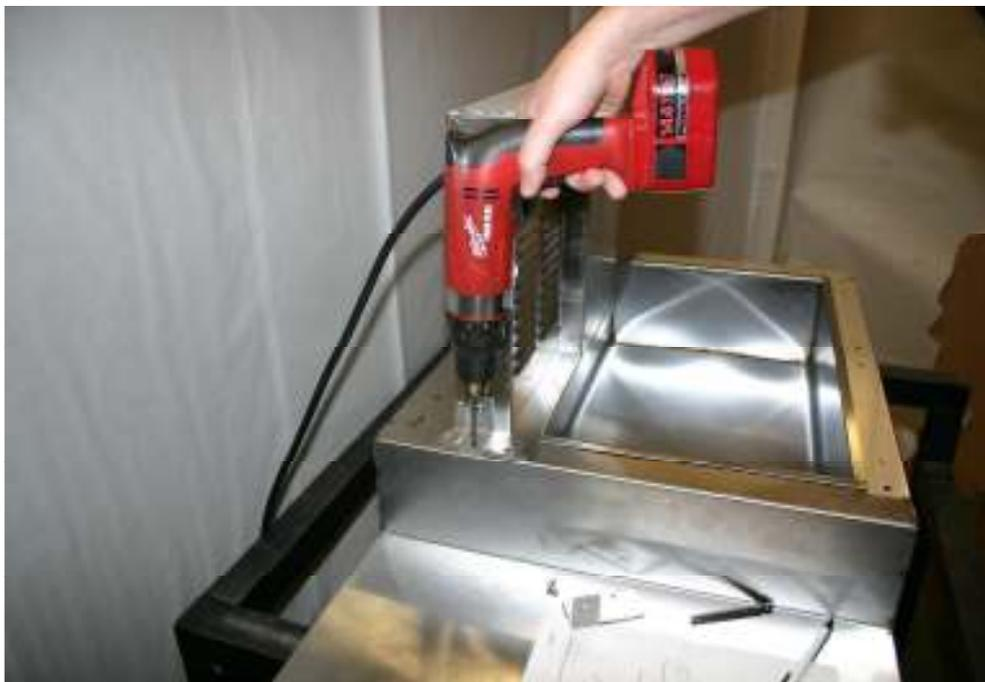
5. Insert and tighten screws provided ([SCR008](#)).
