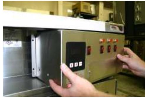
3. Depending on whether the Right Side well or the Left Side well is to be disabled, remove the power wires from the back of the power switch for that well. This would be wires #1 and #2 for the Left Side or wires #5 and #6 for the Right Side. Using the male connectors provided (F0243), cap these wires individually creating a dead end on each wire.
