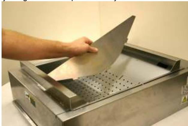
4. Remove the Pan by picking up on the front then lifting entire pan vertically.
