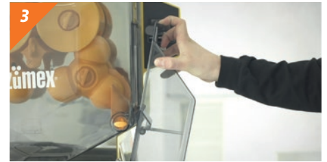
3 Take out the cover sides. Turn the lock / extract the peel guides.
